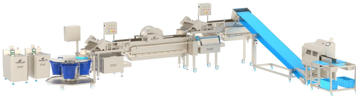
BCM-1650 in a vegetable processing line for cutting, washing and drying vegetables
